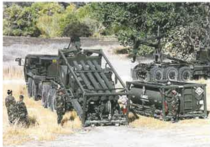
▲ Oshkosh Heavy Mobility Expanded Tactical Truck with Palletised Bulk Fuel Handling Equipment
