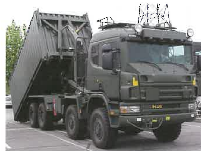
▲ Integrated Load Handling System fitted to Scania P124 CB8x8HZ 420 loading ISO container
