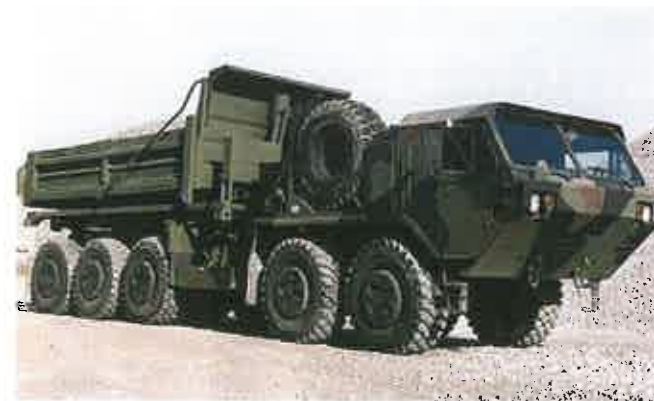
▲ Oshkosh Heavy Mobility Expanded Tactical Truck with Task Specific Module (dump tray)
